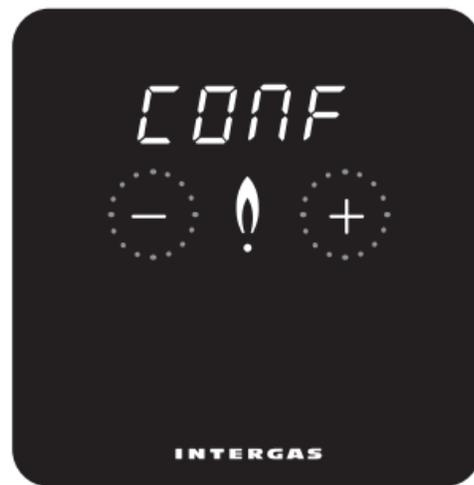
Touch '+' and '-' buttons simultaneously for 2 seconds to open control panel and adjust thermostat settings, if required. Step through menus by tapping '+' or '-' buttons. Confirm selections by tapping centre dot.
