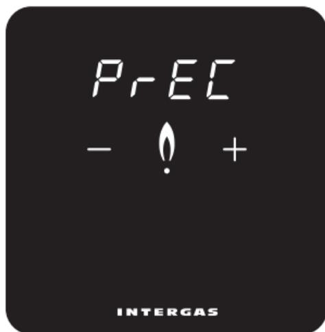
'Tap '+' or '-' buttons to change the way the measured room temperature is displayed. **0,1:** The measured room temperature is displayed in 0,1 °C. **0,5:** The measured room temperature is displayed in 0,5 °C
