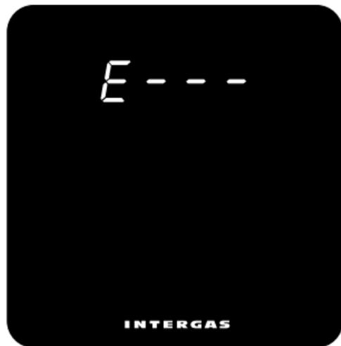
If an "E" with numerical code appears, there is a hardware error in the thermostat. The thermostat will restart after 5 seconds. If this error persists, the thermostat is defective and must be replaced.
