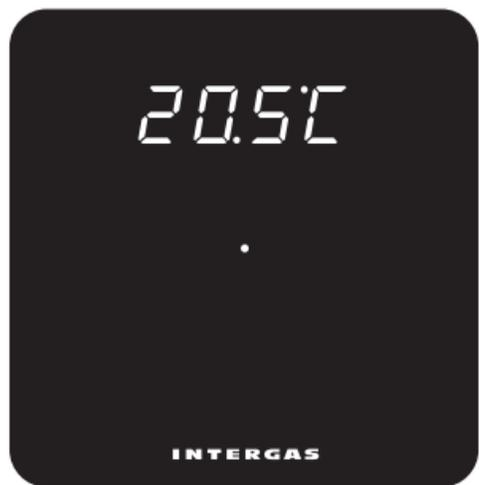
Boiler is in standby, no heat required.
