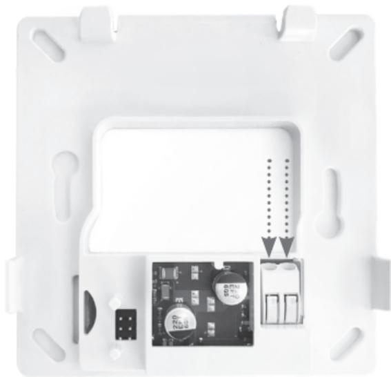
Insert both wires into connector (either way around).
