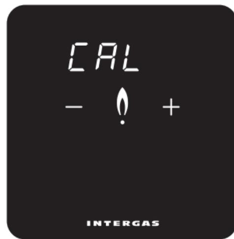
Tap '+' or '-' buttons to correct measured temperature by up to +4 or -4 °C respectively, in increments of 0.1 °C. Displayed temperature may not correlate to actual room temperature, e.g. due to thermostat's position in room. Calibrate to compensate for this effect.
