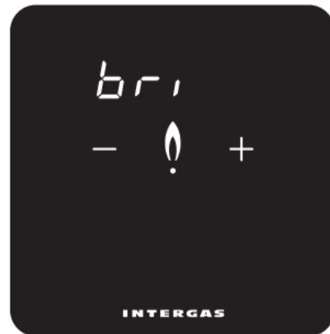
Tap '+' or '-' buttons to adjust thermostat display to desired brightness level. Ten brightness levels available (max. brightness level: 10).
