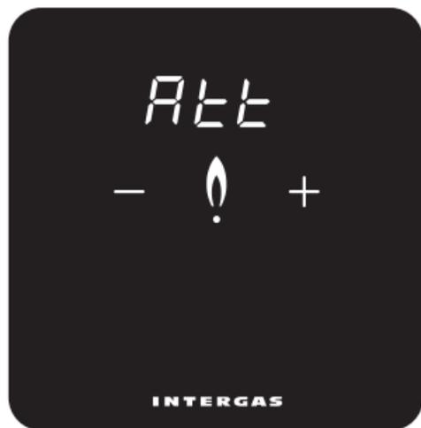
Set display to illuminate when adjusting temperature remotely. Only applies when using Comfort Touch app.
