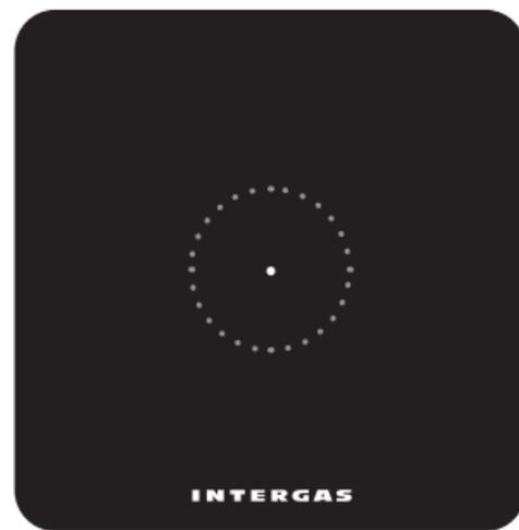
Activate cleaning mode (temporary screen lock) by touching dot for 2 seconds. Clean thermostat screen.
